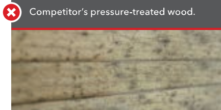
Stain mold present after 7 months of field-testing a competitor's pressure-treated wood. 1
